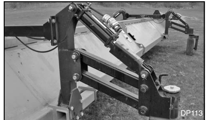
Figure 27. Pivot Tube Lubrication Points
